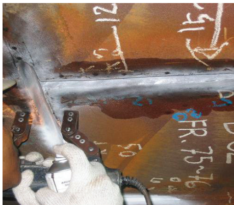
Magnetic particle inspection using a yoke.
