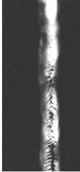
X-ray of a welded seam showing porosity.
